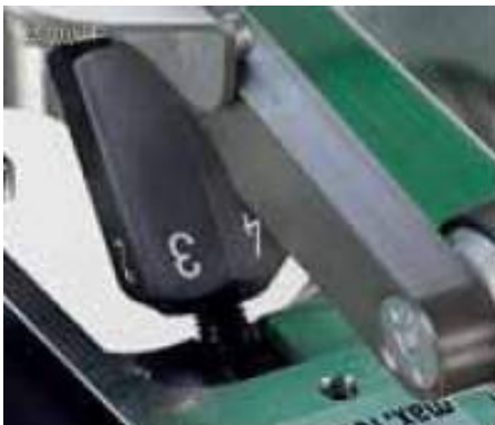
Adjustment of welding force for different materials
