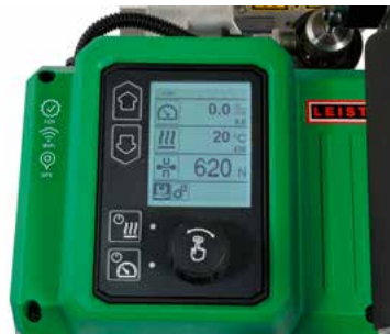
Digital display of welding pressure and voltage
